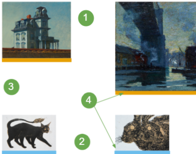
Figure 2: The correct output for the task. Each number refers to the step number. (1) creates and renders the 4 images. (2) puts the images in 2 rows. (3) arranges images by a user-defined property using the arrangeBy method. (4) requires the user to set a label on their data, such that elements with the same label will have a matching stripe along the bottom of the picture.
